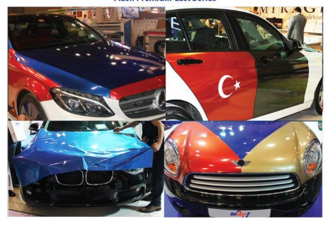
Unicast 9600 flash cast PVC films which have double layer structure and premium color pigments are produced for all 3D surfaces and a full color change applications of the vehicles.
